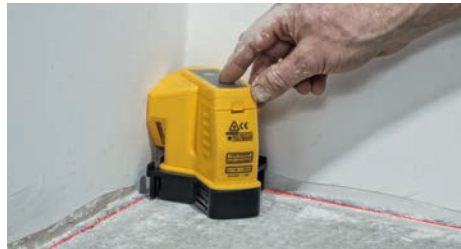
Position inside corner to check for square.
